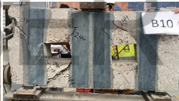
B10-SO-F: Diagonal-shear, concrete cover splitting
