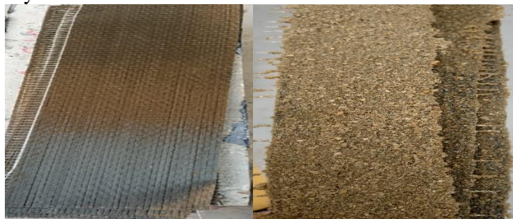
Figure (1): Basalt fiber before and after roughing its surface with sand
