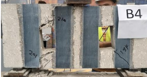
B4- RO-V-F :Diagonal-shear splitting failure
