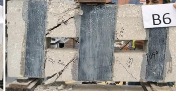
B6-RO-H-F : Diagonal-shear splitting
